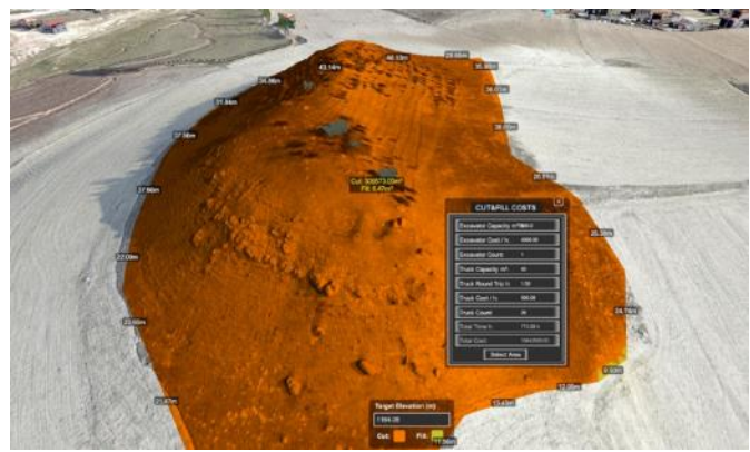
Figure 17 Cut & Fill Cost Analysis
