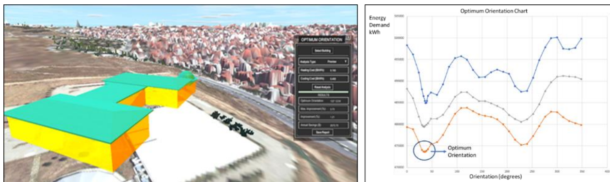
Figure 19 Optimum Orientation of a Building (left) and Optimum Orientation Chart (right)
